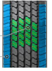
Optimized block edge elements in combination with deep snow sipes provide excellent grip and safe feeling in all road conditions.
